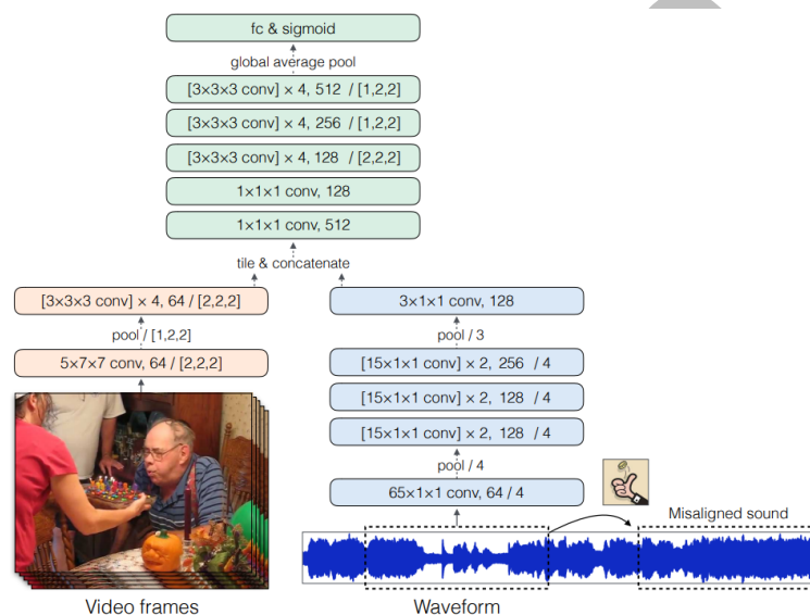
Figure 1: Proposed neural network model by Owens and Efros (2018). Using a fused multisensory representation, they state that a video signal's visual and audio components should be modeled jointly.
